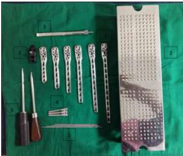
Fig 1: Philos instruments-(1)5,6,7,8,10,12 hole philos plate, (2) locking and cortical screws, (3) depth gauge, (4) drill sleeve, (5) drill bit, (6) locking and non locking screw driver, (7) sleeve guide
