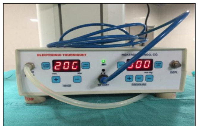
Fig 2: Modern pneumatic Tourniquet system
