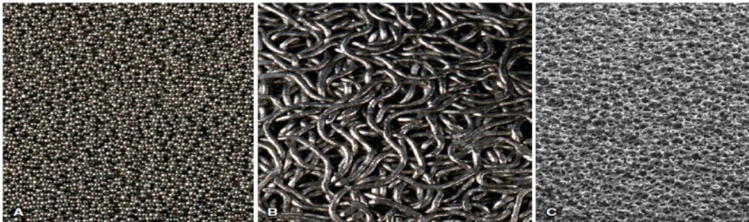
A. Sintered beads B. Fibre mesh design C. Hydroxyapatite crystal coated design.
