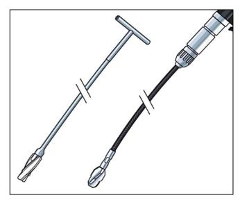
Fig 2: Flexible Reamers
